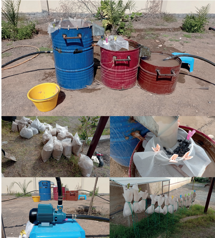
FIGURE 9. The flotation machine built at Fulayj. The water is recycled and recirculated via a domestic pump (left). The sediment is poured into the main barrel and the carbonized macro-botanical remains are gathered in a fine mesh (right) before being air dried (bottom).
